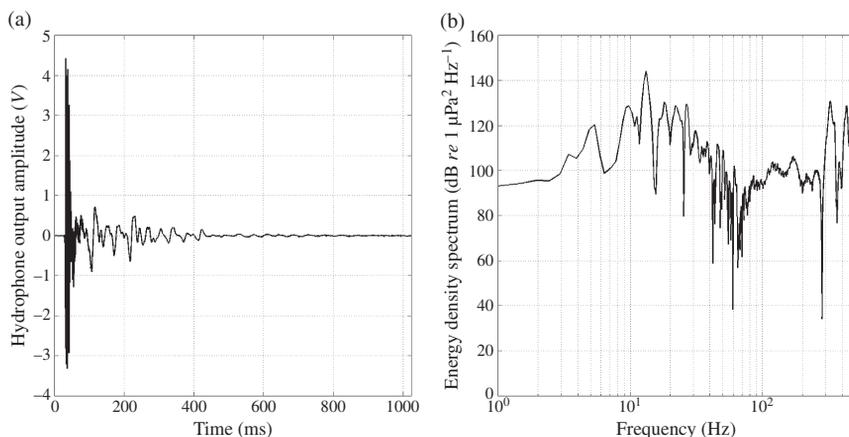
FIG. 1. (a) Representative time series of amplitude of a single airgun blast. In total, there were 50 blasts with *c.* 10 s between blasts. (b) Energy density spectrum representative of a single airgun blast of the signal shown in (a).
